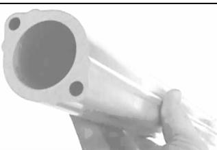
Profiles with cavities (known as "Hollows") can be produced to eliminate milling. If the current raw material "Blank" is made from plate stock and then milled or laser cut (or even water cut) to achieve and interior and or exterior shape. An extrusion can be produced to eliminate the requirement of milling the interior and exterior, one only needs to CNC cut the desired thickness from the linear extruded profile to obtain the product.
